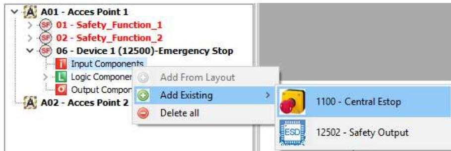
1. Add the Input elements to the Safety Function using the Manual Mode
