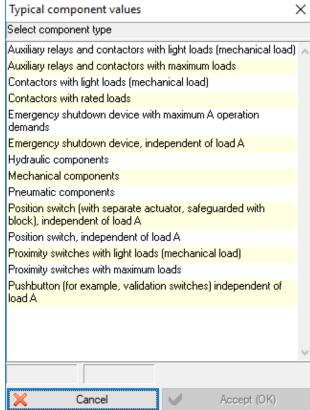
5. If the B10d value of the element is not known, click on "typical components values", and select the component type.
